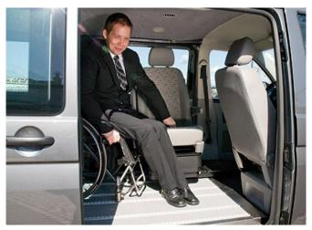
The **6-way Base** is a swivel seat system that enables an easy transfer from the wheelchair into a safe and secure front driver or passenger position in the vehicle. Suited for vehicles with a flat floor entry into the front seating positions the **6-way Base** allows the driver to move forwards, backwards, rotate to 1400 degrees, as well as moving up and down to match the height of your wheelchair.
