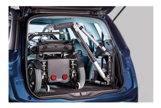
The Smart Lifter is a hoist that enables a mobility device, such as a wheelchair, scooter or powerchair, to be easily and simply lifted into a car boot at the touch of a button. This eliminates the need for the wheelchair/scooter user or family member to struggle with getting the device into a vehicle when wanting to venture further afield.
