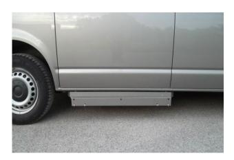
The **Autolift F6 Underfloor Lift** is a fully automatic underfloor cassette lift designed to transfer a wheelchair occupant in and out of the vehicle. It features a robust cassette that is installed underneath the vehicle meaning you can utilize the full space inside of the vehicle for passengers and luggage!
