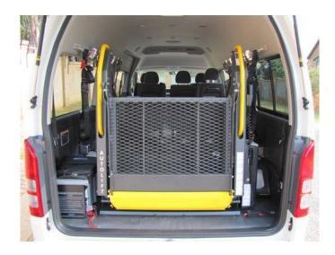
Horizontal split twin pillar hydraulic platform lift
